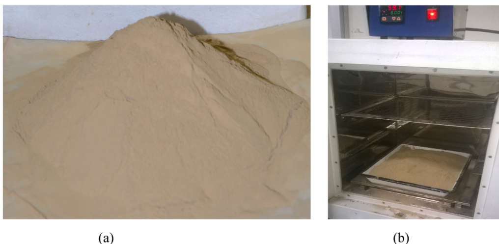
Fig. 1. (a) Barmer bentonite clay used in the study and (b) thermostatically controlled oven for heat treatment.
