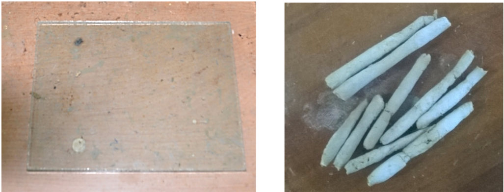
Fig. 3. (a) Smooth glass plate for plastic limit test and (b) rolled samples.
