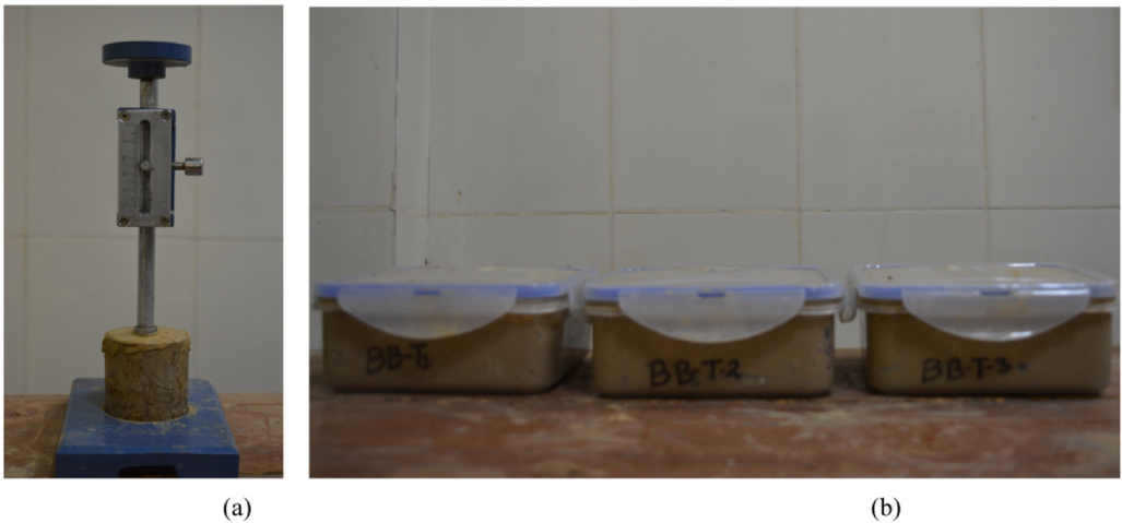
Fig. 2. (a) Liquid Limit testing apparatus and (b) sealed container for sample preparation.
