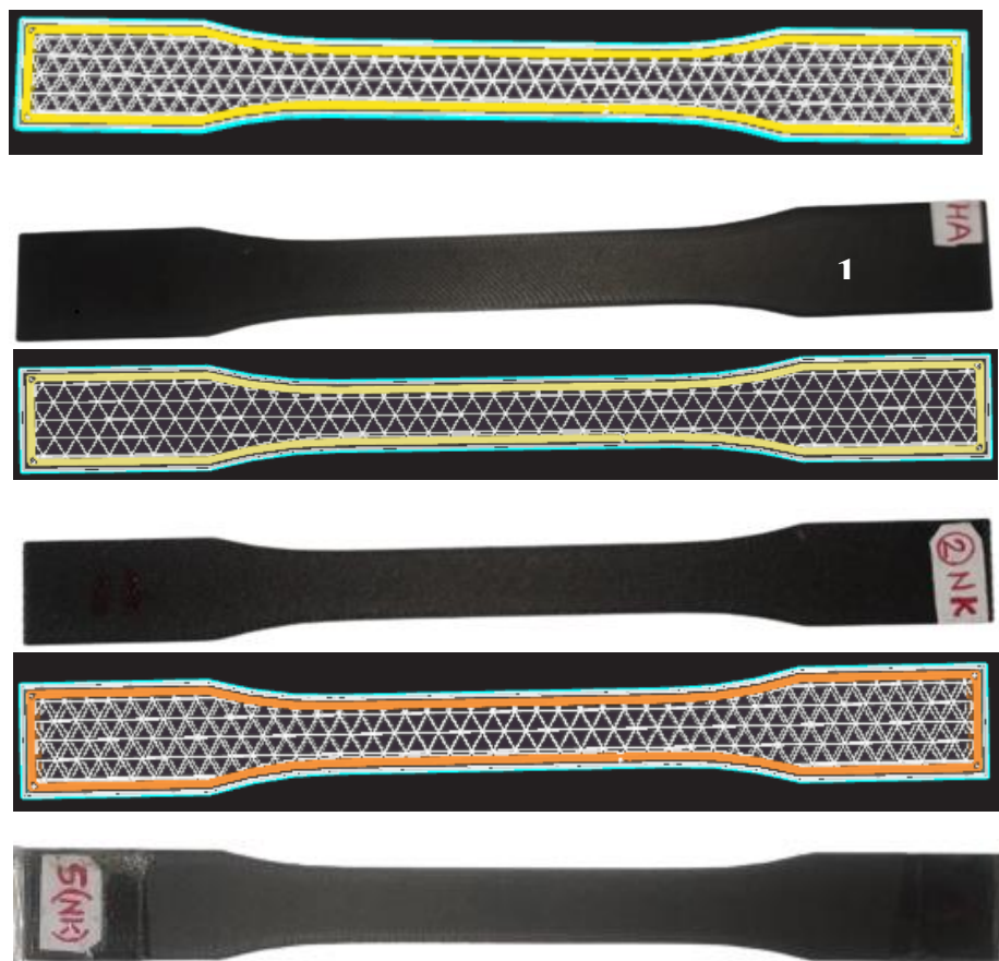
Figure 3.4. Tensile Specimen dimension as per standards ASTM D 638 type-I where 1-KFRT, 2-GFRT and 3-HSHTRT yellow lines represents the fiber filaments and others are matrix (nylon).
