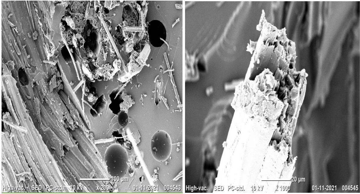
Figure 3.25. SEM micrograph of bending fracture surface of cross specimen
