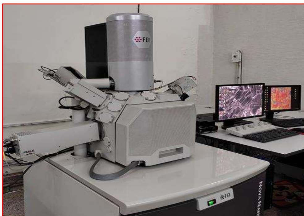
Figure 2.4 Scanning electron microscope (Model: Nova Nano SEM 450).
