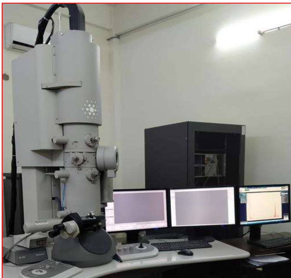
Figure 2.3 Transmission electron microscope (Model: Tecnai G2 20 TWIN).
