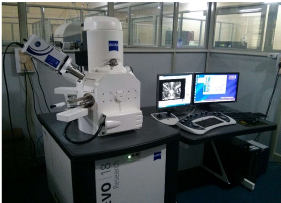
Figure 2.9. FESEM facilities at Central Instrument Facility (CIF) IIT (BHU).
