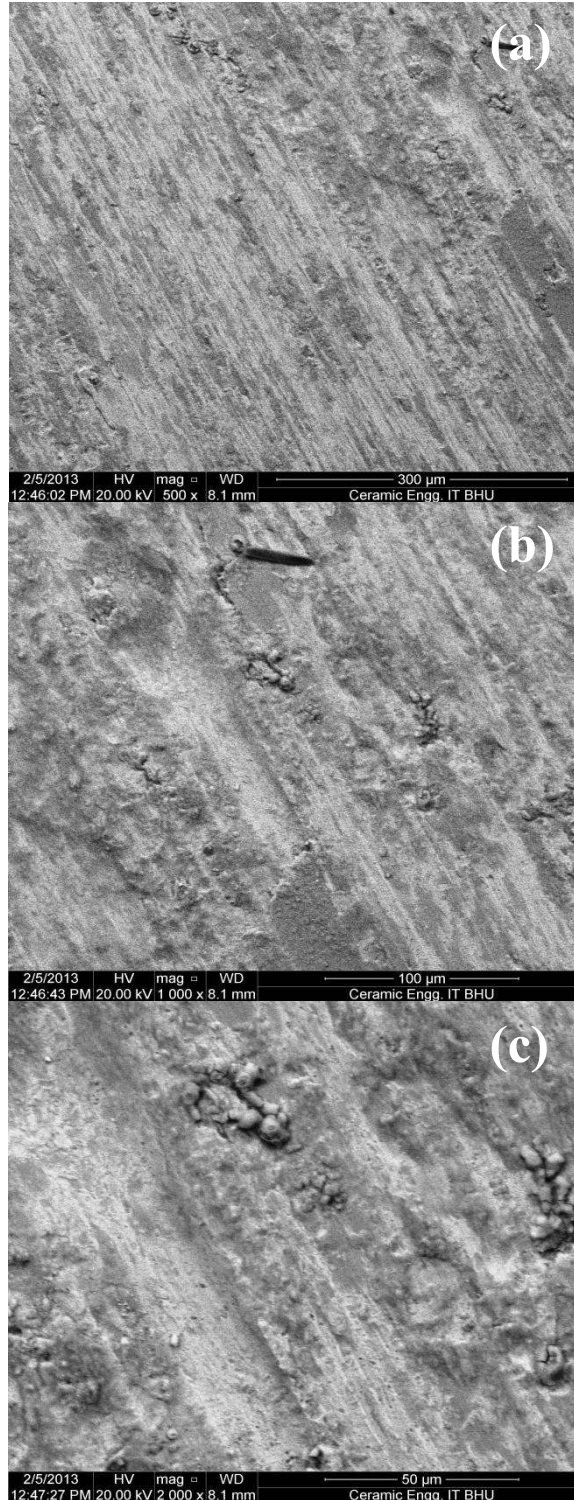
Fig. 8.37 Microstructure of the worn specimen 3.5Zr1.5AlFe1000(2) after 2.0 Kg load at (a) 500X (b) 1000X and (c) 2000X magnification respectively
