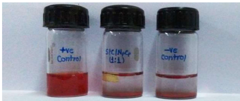
Fig 6.14 Visual confirmation haemocompatibility of S/C/NpCp (1:1) by hemolytic activity shown by sample after incubation in physiological saline at 37°C for 1h
