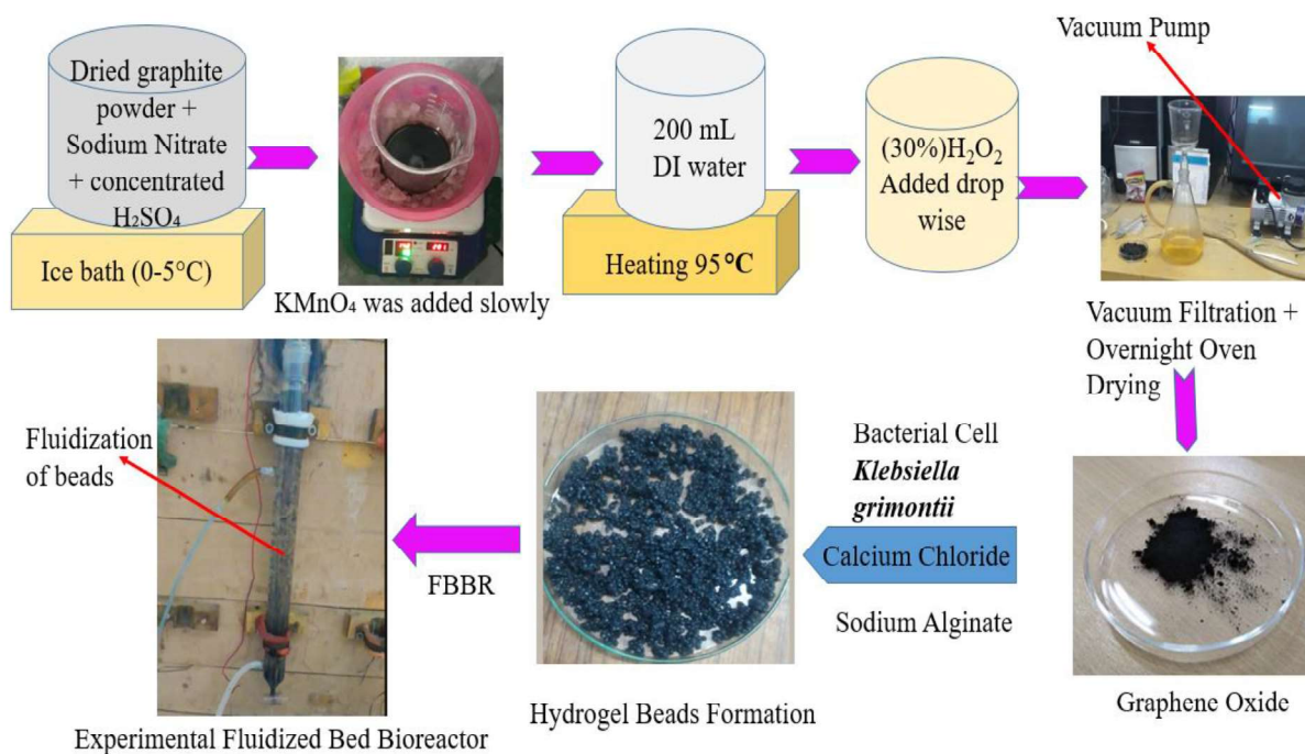
Figure B-2. A schematic layout of Graphene Oxide Preparation strategy with hydrogel beads formation and subsequently AB 113 biodegradation in laboratory-scale Fluidized Bed Bioreactor.
