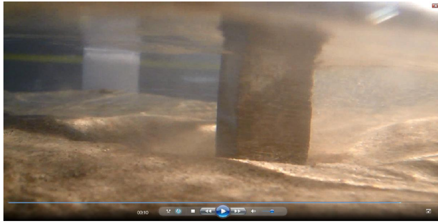
(d) Visualization of vortex motion around rectangular slender structure at time 0.10 sec
