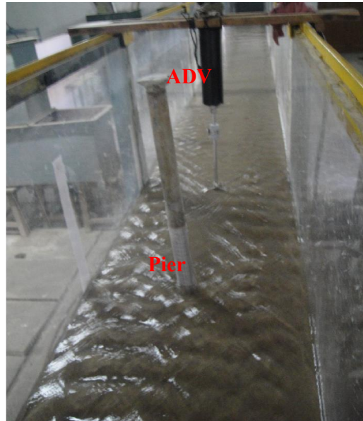
Figure 3.6: Acoustic Doppler Velocity (ADV) setup
