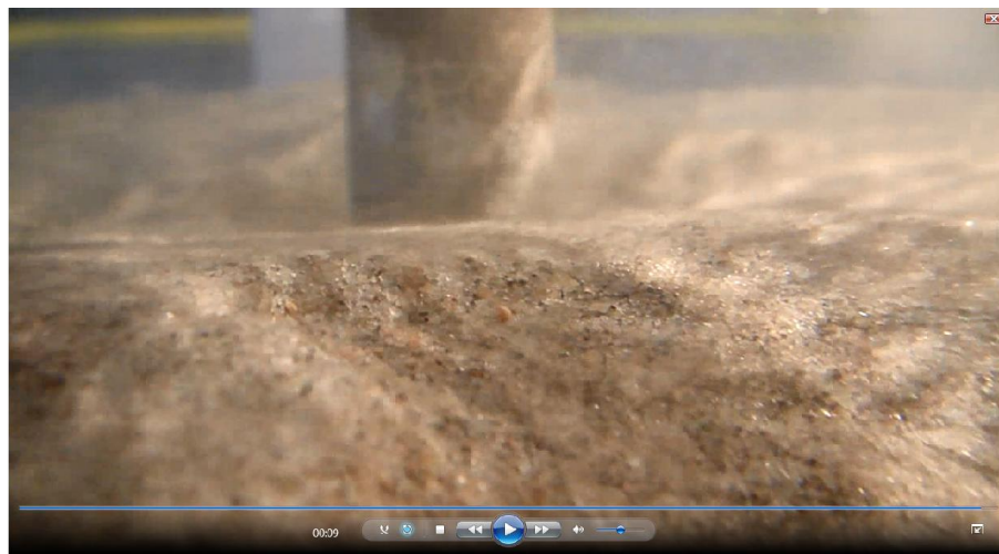
(d) Visualization of vortex motion around cylindrical slender structure at time 0.09 sec
