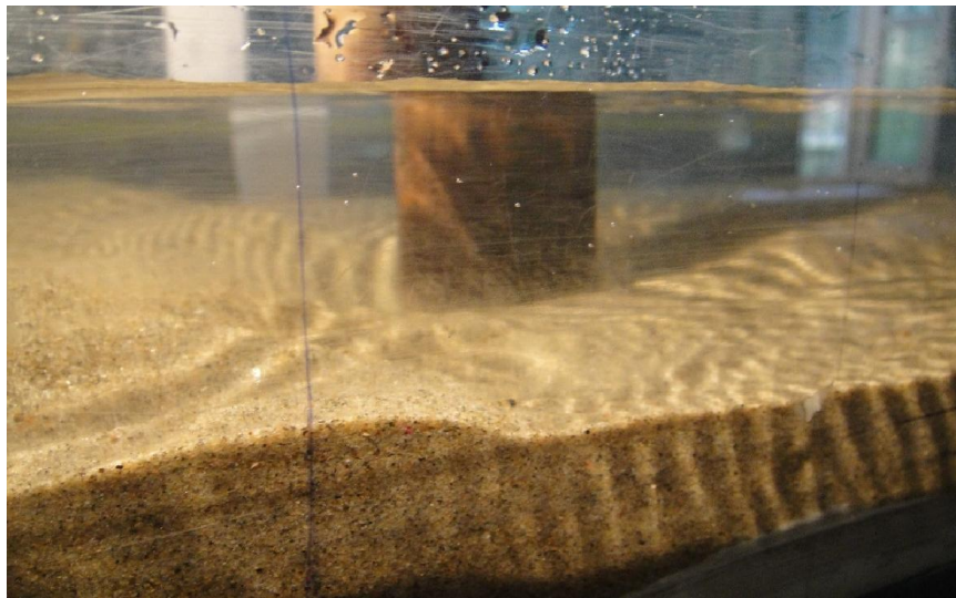
(c) Visualization of vortex motion around oval slender structure at time 0.08 sec
