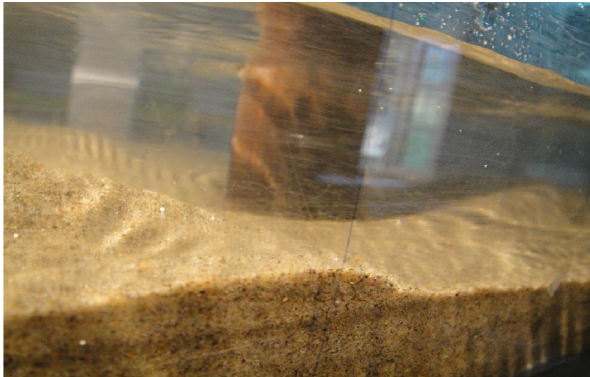
(b) Visualization of vortex motion around oval slender structure at time 0.04 sec
