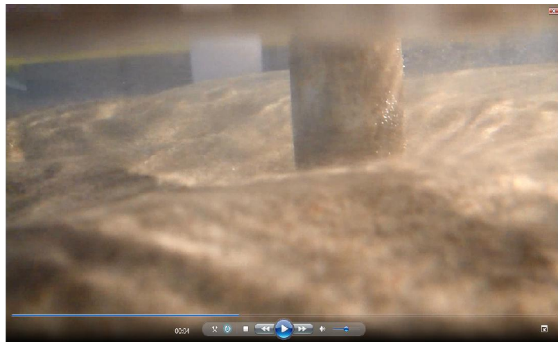
(b) Visualization of vortex motion around cylindrical slender structure at time 0.04 sec
