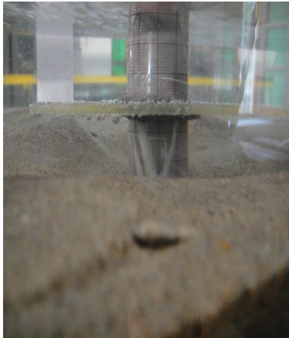
Figure 3.41: View of scour hole around circular pier fitted with collar
