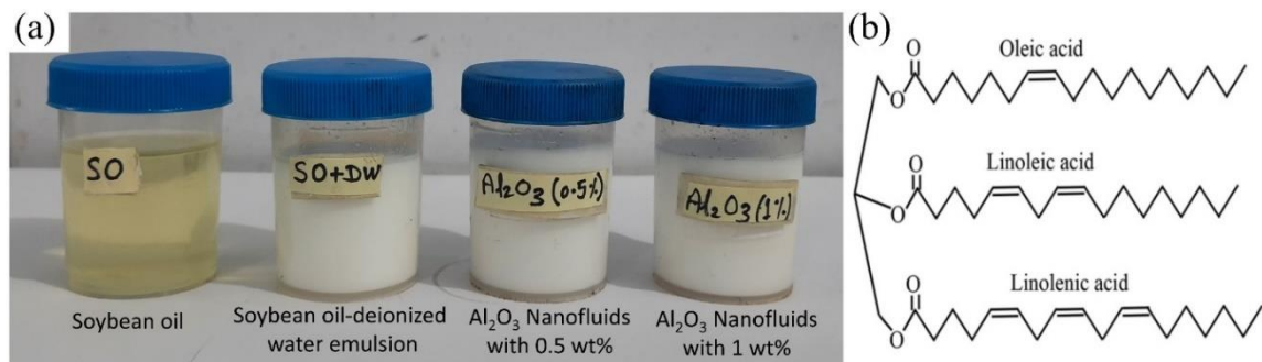
Figure 6.1 (a) Prepared eco-friendly cutting fluids used in UVAMQL grinding, (b) Molecular structure of soybean oils
