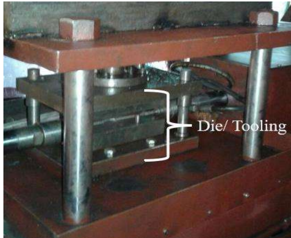
Figure 1.1.2: Die/Tooling attachment system [8]
