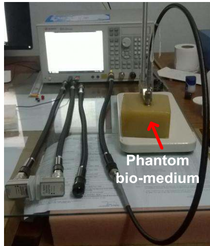
Figure C.1: Experimental setup for measuring the permittivity of prepared biological phantom.
