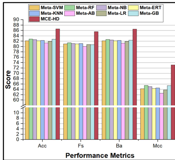
Figure 6.9: Comparison of results obtained by meta machine learning models and our proposed framework (MCE-HD).
