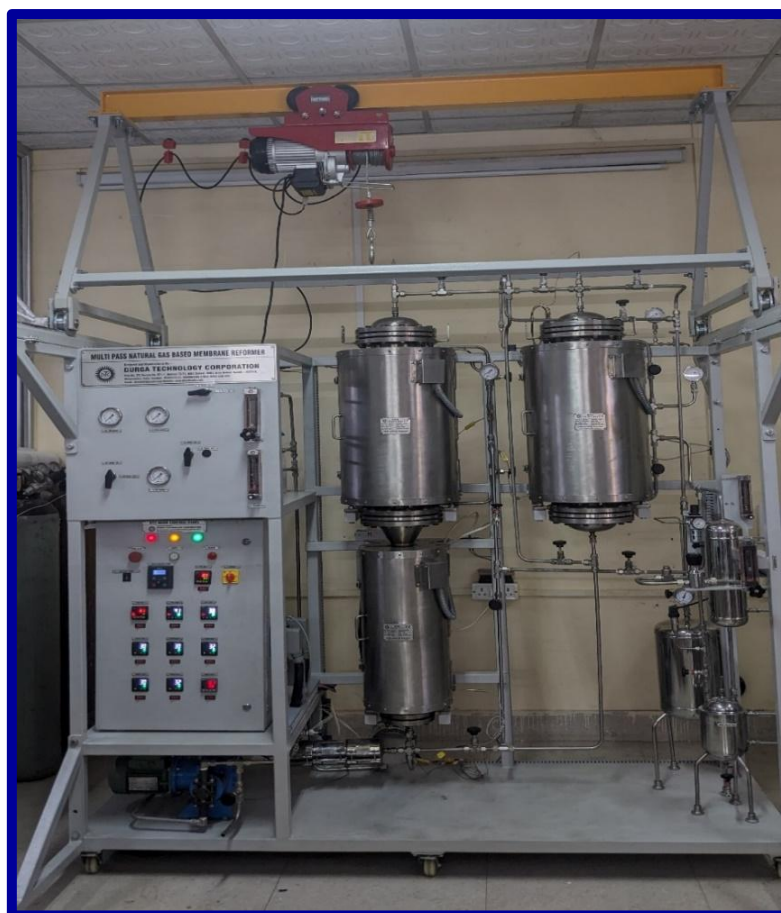
Fig. 6.1 Experimental set up of scale up reactor of I.D 6.35cm
