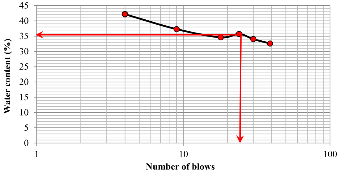
Fig. 5.4. Flow curve of local soil for the determination of liquid limit.
