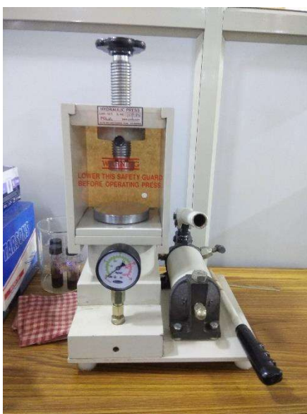
Figure 2.3: Experimental setup of hydraulic press machine
