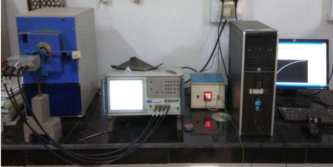
Figure 2.15: Experimental set up of automated impedance analyzer along with sample holder and furnace (6500 P Wayne Kerr, UK)
