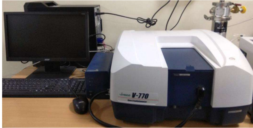
Figure 2.12: Experimental setup of UV-Visible measurement [JASCO V-770 UV-Vis spectrometer].
