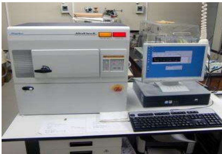
Figure 2.7: Experimental setup of X-ray diffractometer [Rigaku Miniflex II]
