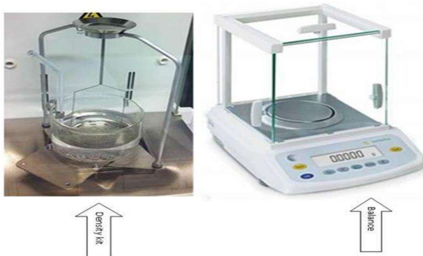
Figure 2.5 Density kit and weighing balance [Sartorius, BSA2245CW]
