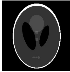
Fig. 2.10: Modified Shepp-Logan phantom ( 128 \times 128 pixels)
