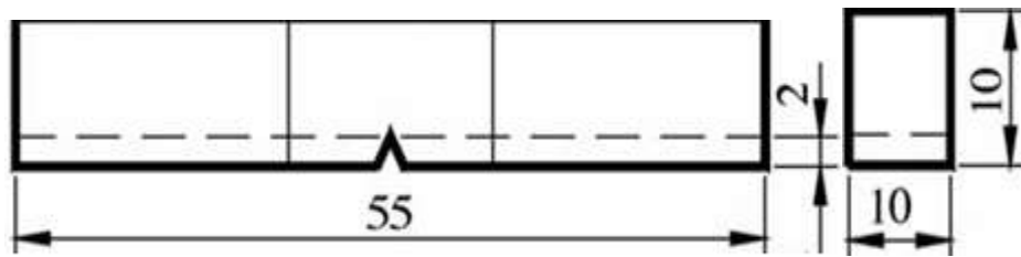
Figure 3.10 Dimensions (mm) of “sub size” Charpy V-notch test samples [88]
