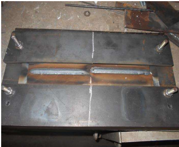
Figure 3.2 AISI 304 plates after welding in Fixture Figure 3.3 AISI 304 plates during welding
