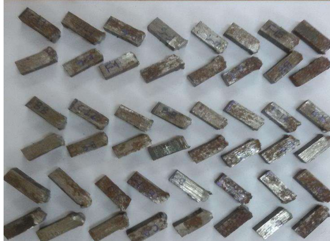
Figure 3.12 Charpy test samples after fracture
