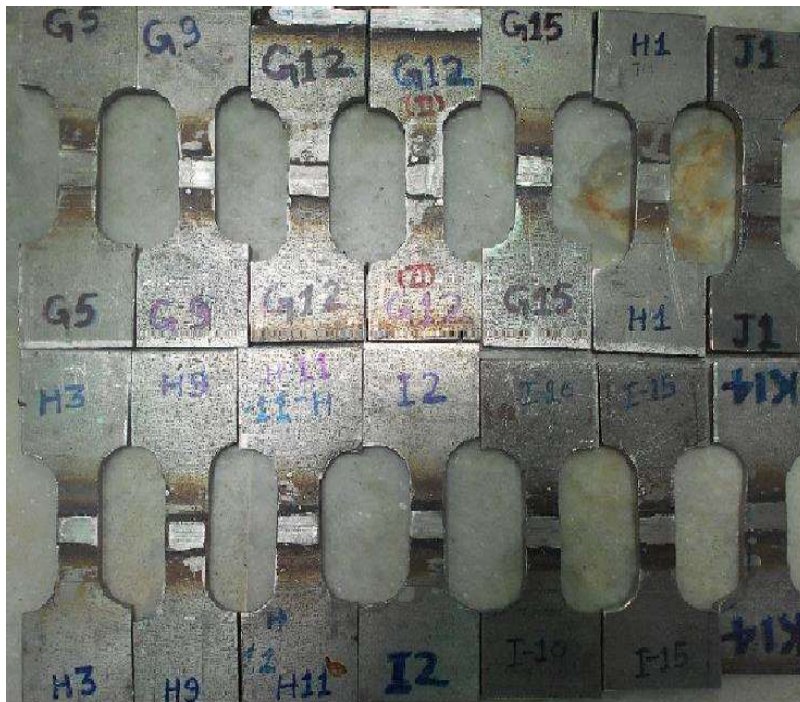
Figure 3.9 Actual photograph for a tensile test of AISI 304
