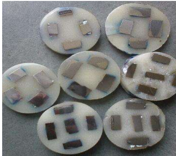
Figure 3.13 Samples for microstructure & Vicker hardness test
