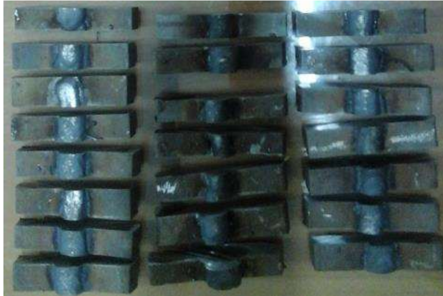
Figure 3.11 Actual photograph for Charpy test samples
