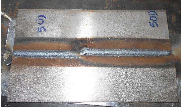
Figure 3.4 AISI 304 plates after weld
