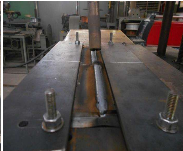
Figure 3.2 AISI 304 plates after welding in Fixture Figure 3.3 AISI 304 plates during welding
