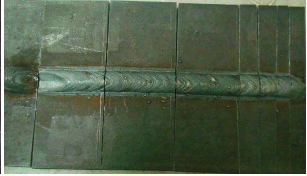
Figure 3.5 IS 2062 welded plate after cutting
