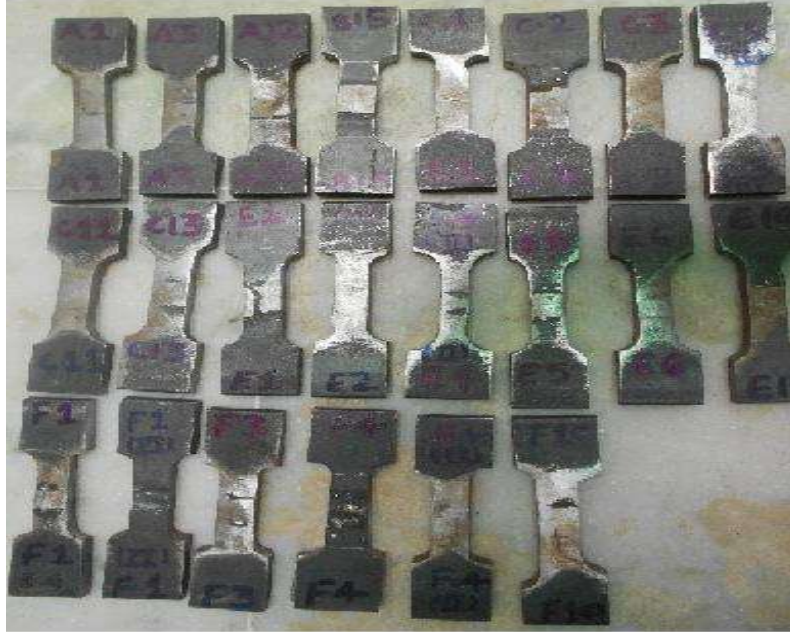
Figure 3.8 Actual photograph for the tensile test of IS 2062 steel
