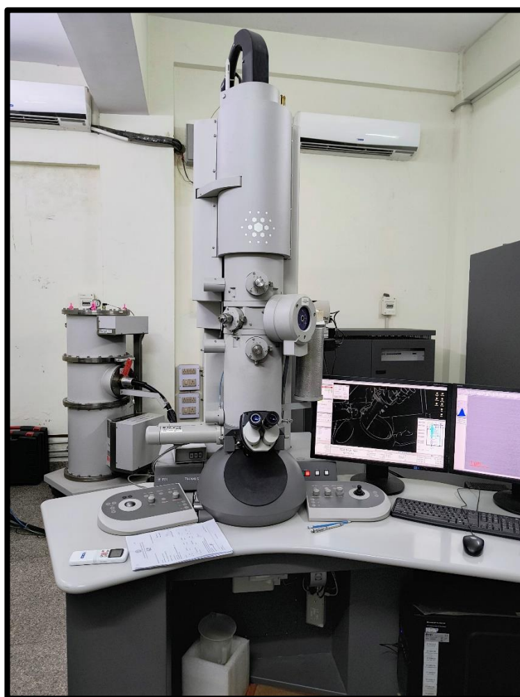
Figure 2.4 Transmission electron microscopy with EDX (FEI, TECHNAI G2 20 TWIN, Courtesy CIFIC IIT BHU).
