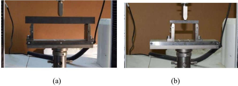
Fig. 4.10 Testing arrangement of flexural specimens having square cross-section applied to three point bend loading (a) Large size and (b) Small size specimen.
