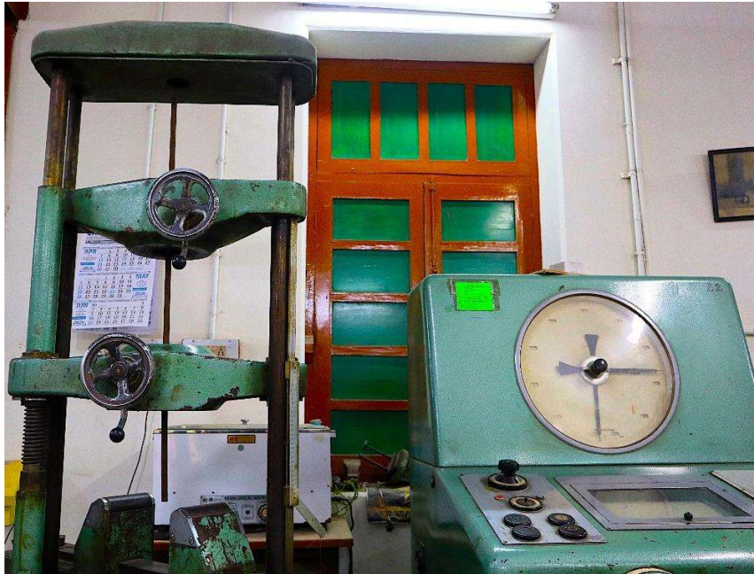
Figure 5.2 UTM set up to measure the tensile strength of a 12 mm bar at Structural Engineering Laboratory, Civil Engineering Department, IIT-BHU, Varanasi
