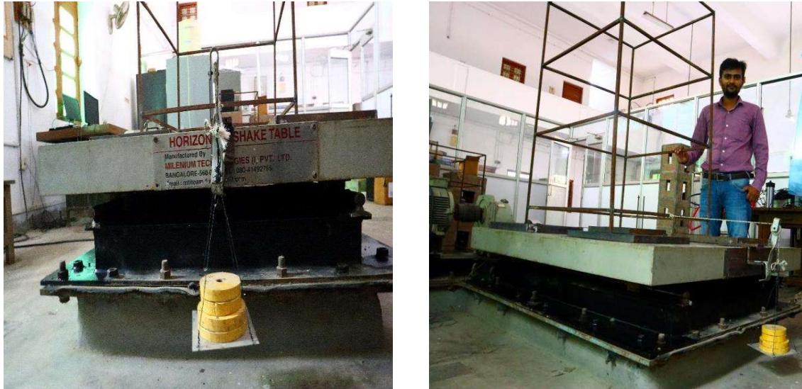
Figure 5.4 String-Pulley laboratory test setup for the calculation of the friction value in a test chamber at the Structural Dynamics Laboratory, Civil Engineering Department, IIT-BHU, Varanasi.
