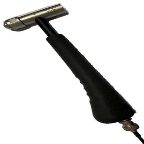
Figure 5.7 Impact hammer type Bruel and Kjaer 8206-003 in Structural Dynamics Laboratory, Civil Engineering Department, IIT-BHU, Varanasi.
