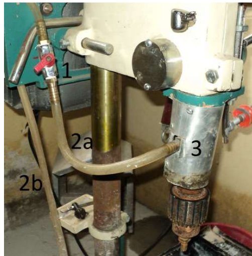
Fig. 3.15: Picture of Fluid Inserting Assembly
