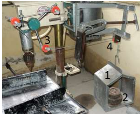
Fig. 3.4: Picture of Pulley Loading Mechanism
