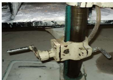
Fig. 3.9: Picture of Platform Adjusting Assembly
