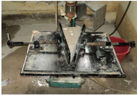
Fig. 3.8: Picture of Jaw Holding Un-Parallel Rock Sample on Drilling Platform
