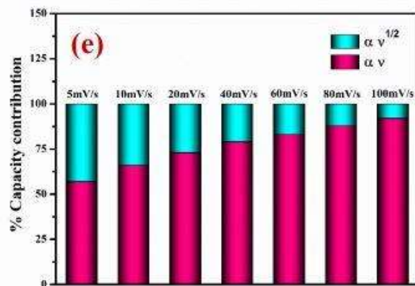
Figure 4.12: (a) \log i_{cp} , \log i_{ap} vs \log v plot, (b) variation of b with applied potential, (c) plot between i/v^{1/2} vs. v^{1/2} , (d) CV at 5 \text{ mV s}^{-1} showing intercalation and surface contribution separately, (e) intercalation and surface contribution at different scan rate, and (f and g) corresponds to the Trasatti plot of \text{K}_{0.4}\text{MnO}_2 \cdot x\text{H}_2\text{O} electrode.
