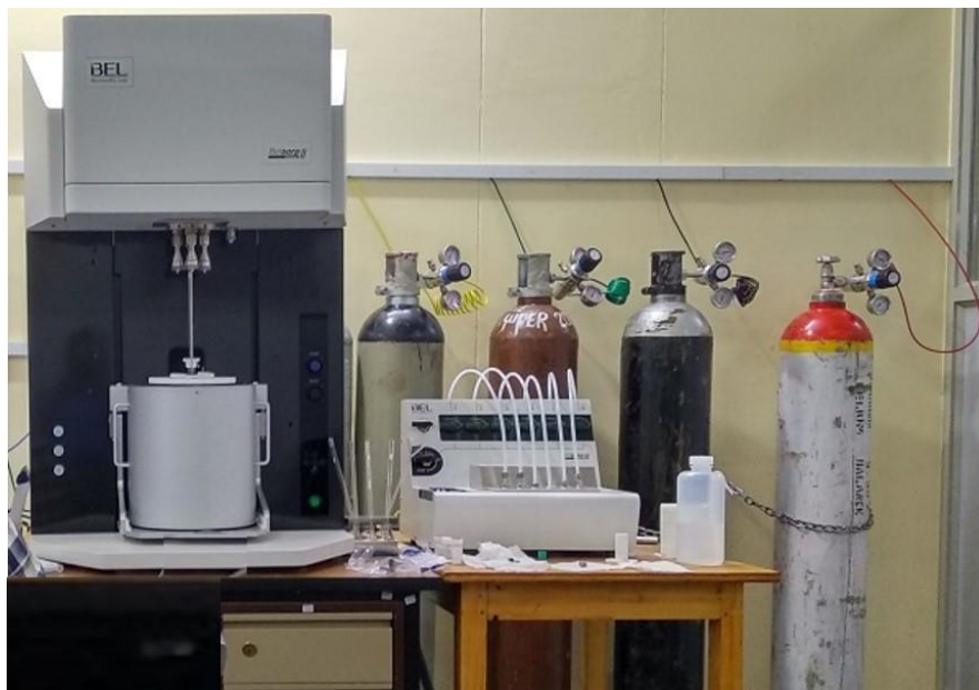
Figure 2.9: Digital photograph of BET measurement setup (CIF, IIT BHU).
