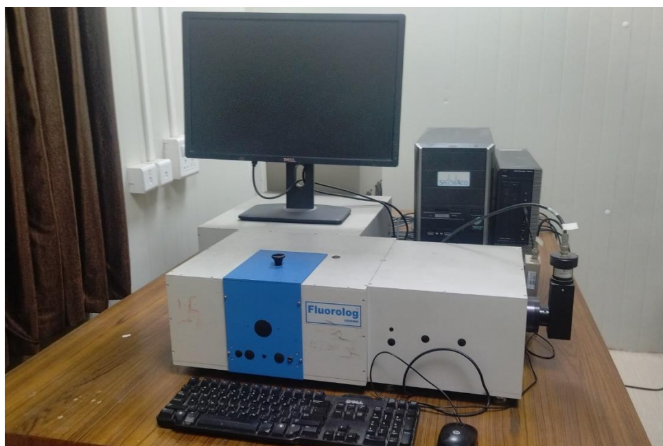
Figure 2.16: Digital photograph of Horiba Fluorolog-3 spectrophotometer (Department of Physics, IIT BHU).
