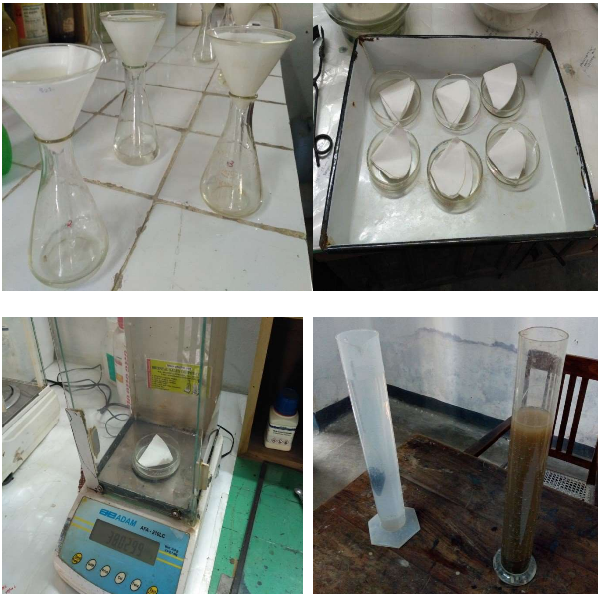
Figure 3.8 Estimation of suspended sediment load in lab
