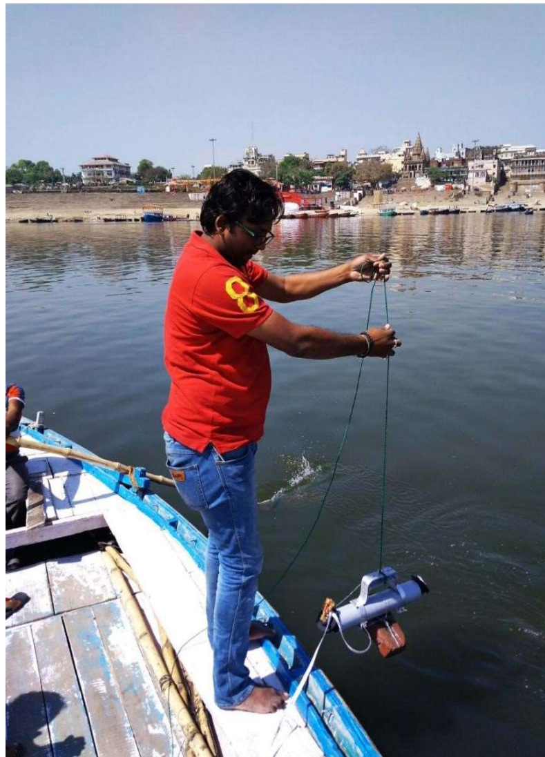
Figure 3.7 Photographic view of water sampling taken for sediment concentration
