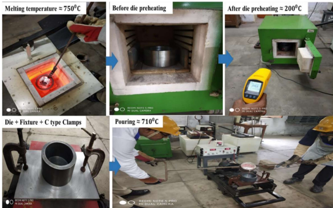
Figure 3.6: Melting, die preheating, die & fixture assembly and pouring
