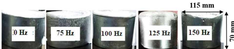
Figure 3.9: Cast components under a high-frequency (0-150) Hz range
