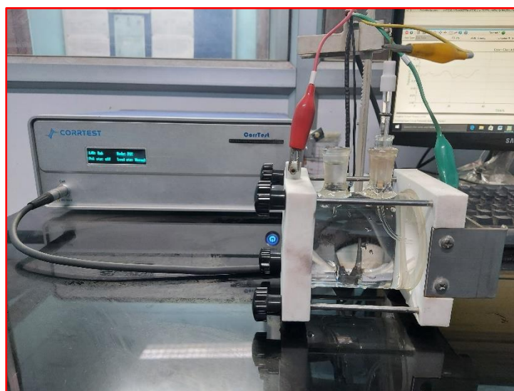
Figure 2.17 Potentiostat with flat cell having three electrode system.
