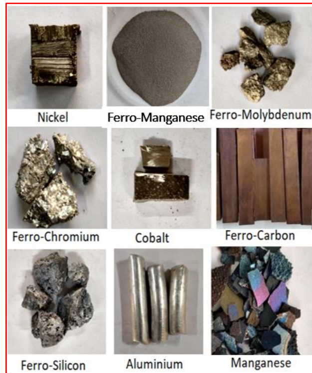
Figure 2.1 Raw materials used for making studied compositions.
