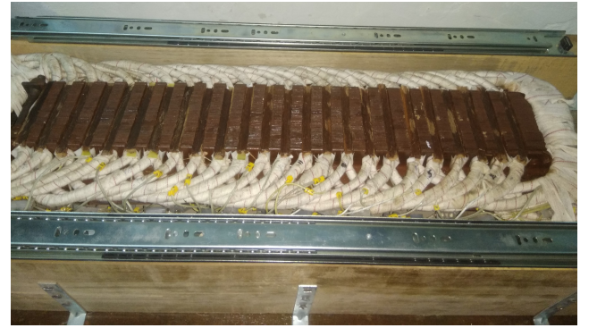
FIGURE 9: Prototype SLIM stator with sliding support for secondary sheet
