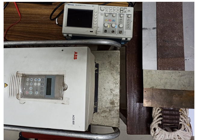
FIGURE 10: Setup for testing of the prototype SLIM
