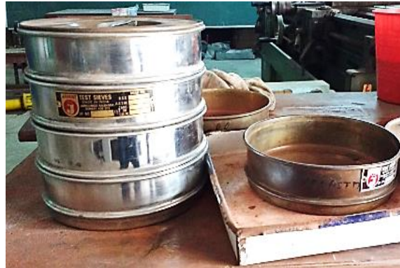
Figure 2.4 Set up used for particle analysis of iron ore
