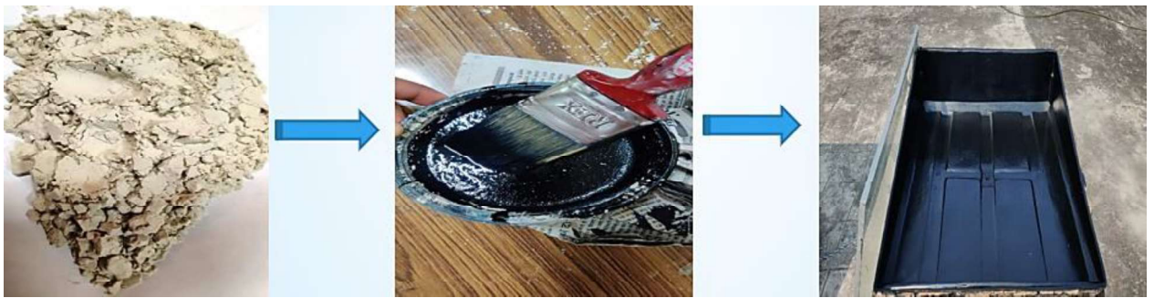
Figure 3. 7 BPQD-black paint mixture coated on solar still
