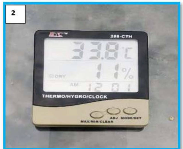
Figure 3. 3 Weather measuring instruments (1). Solar power meter (ISO 9001:2008) (2). Digital thermometer
