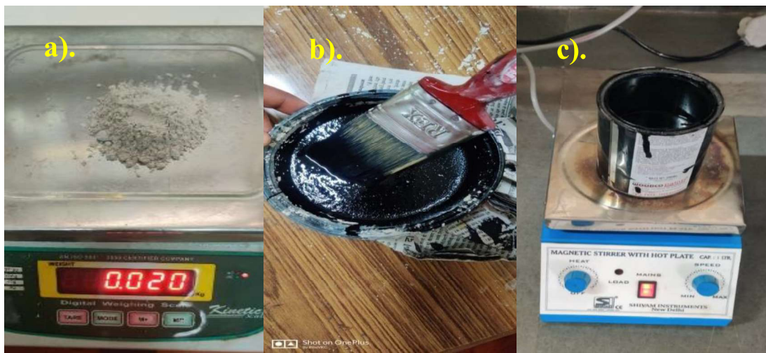
Figure 3. 5 Preparation of coating material a). weighted BPQD b). QD with black dye c). Mixing by Magnetic stirrer
