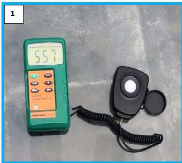
Figure 3. 3 Weather measuring instruments (1). Solar power meter (ISO 9001:2008) (2). Digital thermometer
