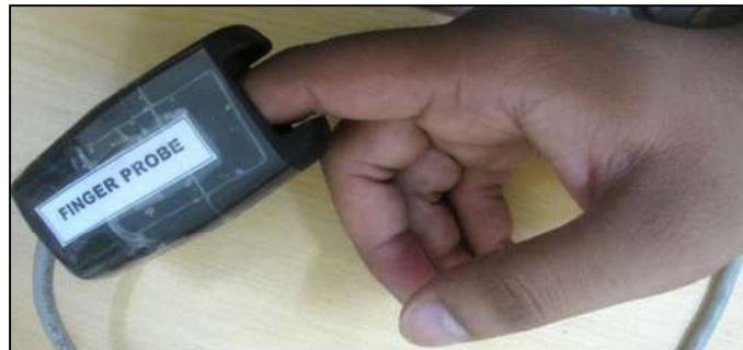
Figure 3.20: Finger holder probe of our noninvasive technique based prototype unit.
