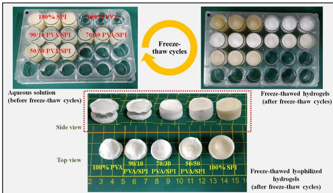
Figure 3.2 Digital images fabricated all FT PVA/SPI hydrogels: before freeze-thawing, after freeze-thawing and after lyophilisation.
