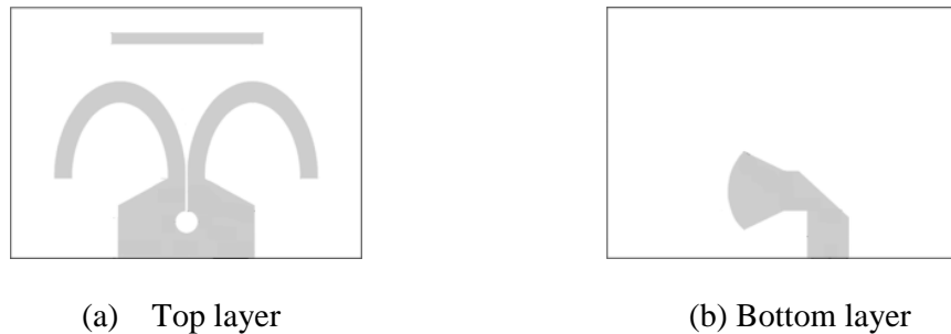
Figure 2.55 Geometry of uniplanar dipole antenna with tapered slot feed and parasitic element
