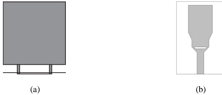
Figure 2.3 Monopole antenna structures with double feed
