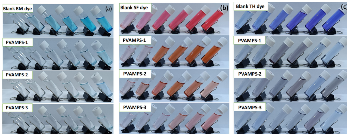
FIGURE 15 This images shows the effect on color of dye solution after adsorption with Synthesized PVAMPS hydrogels (PVAMPS-1 ( 1.25 \times 10^{-4} mol/L of poly (vinyl alcohol) and 2.41 mol/L of AMPS)), PVAMPS-2 ( 0.62 \times 10^{-4} mol/L of poly (vinyl alcohol) and 3.62 mol/L of AMPS) and PVAMPS-3 ( 0.31 \times 10^{-4} mol/L of poly (vinyl alcohol) and 4.82 mol/L of AMPS), (a) changes in appearance of MB dye after adsorption by PVAMPS hydrogels, (b) changes in appearance of SF dye after adsorption by PVAMPS hydrogels, (c) changes in appearance of TH dye after adsorption by PVAMPS hydrogels. [Color figure can be viewed at wileyonlinelibrary.com ]
