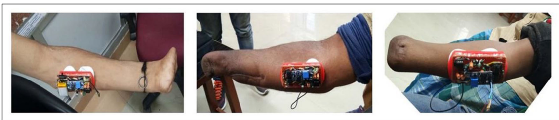
Fig. 2 EMG sensor attachment on residual forearm stump of amputees
