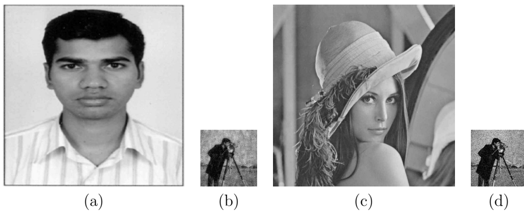
FIGURE 7.10: (a, c) Watermarked of Photo and Lena Images after JPEG Compression(Q=30)( b, d) Extracted watermarks
