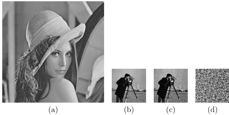
FIGURE 7.17: (a) Watermarked Image; (b) Watermark Image; (c) Extracted watermark with entering valid Keys and parameters of Arnold Cat Map; (d) Extracted watermark with entering fake Keys and parameters of Arnold Cat Map
