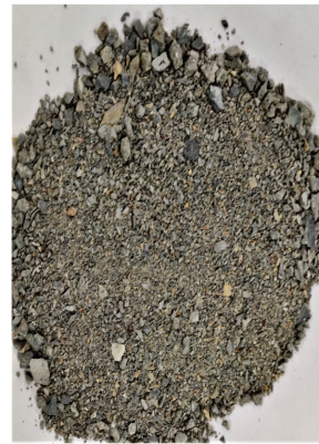
(h) F-RCA (Recycled fines)
