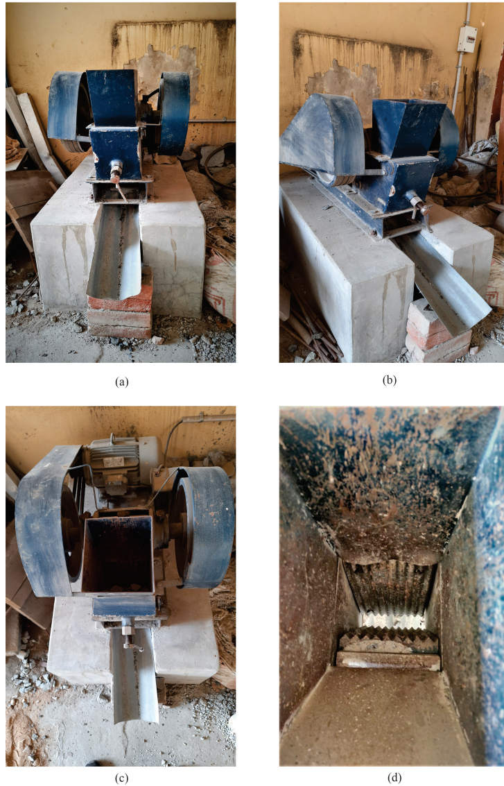
Figure 4.1: Jaw crusher used for crushing the concrete waste. (a) Front view (b) Side view (c) Top view (d) Jaw opening.
