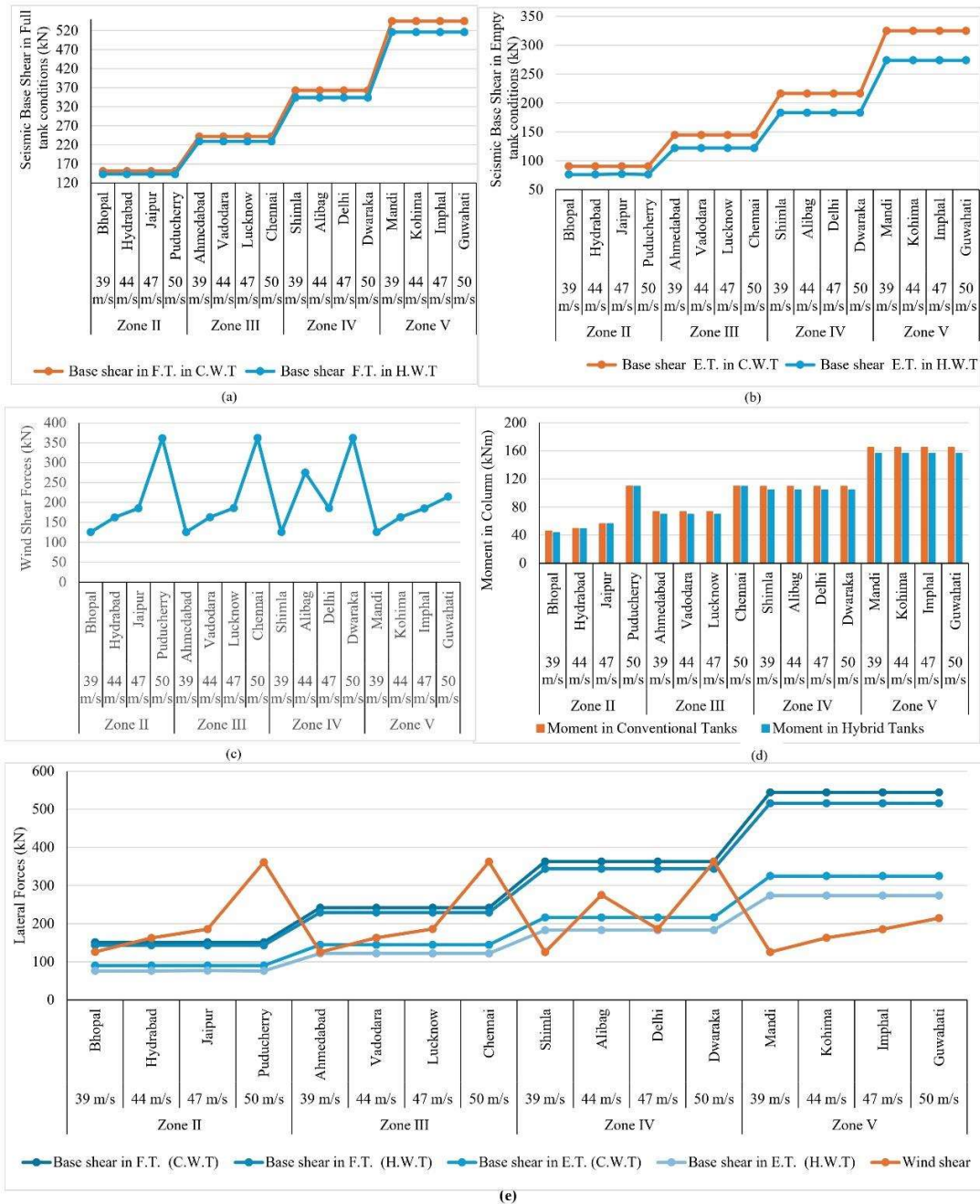
Fig. 6.5 (a) Seismic base shear in Full tank conditions; (b) Seismic base shear in Empty tank conditions; (c) Wind shear forces acting on tanks in 16 cities; (d) Bending moment in columns; (e) Comparative analysis of Base shear forces & wind shear forces in Full & Empty tank conditions across 16 cities.
