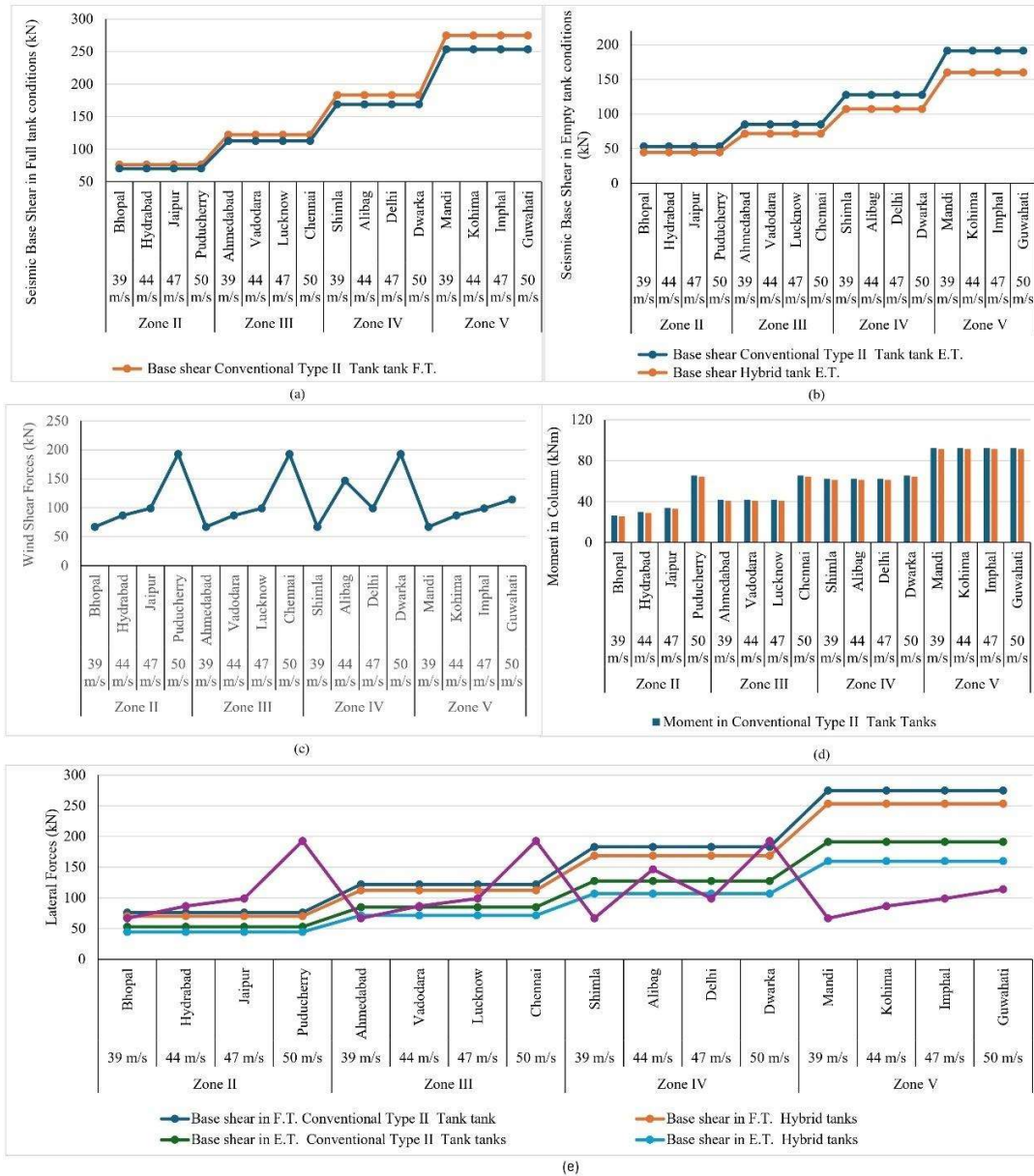
Fig. 6.9 (a) Seismic base shear in full tank conditions; (b) Seismic base shear in empty tank conditions; (c) Wind shear forces acting on tanks in 16 cities; (d) Bending moment in columns; (e) Comparative analysis of base shear forces & wind shear forces in full & empty tank conditions across 16 cities.
