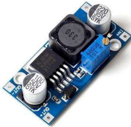
Figure 2.11 DC-to-DC Buck Converter
