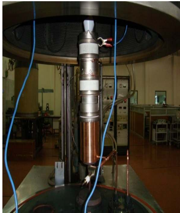
Fig. 3.11: Vacuum processing of MIG at BEL, Bangalore.
