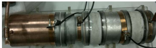
Fig. 3.13: Vacuum processed MIG.
