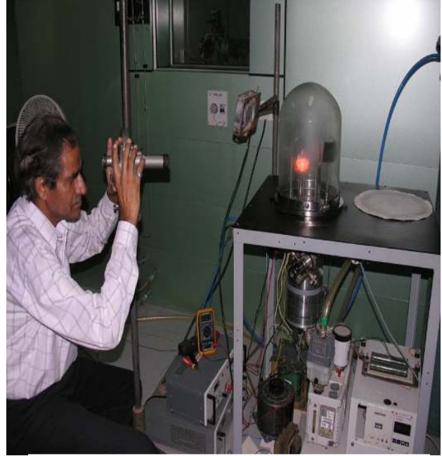
Fig. 3.9: Temperature measurement of cathode in the bell-jar system.
