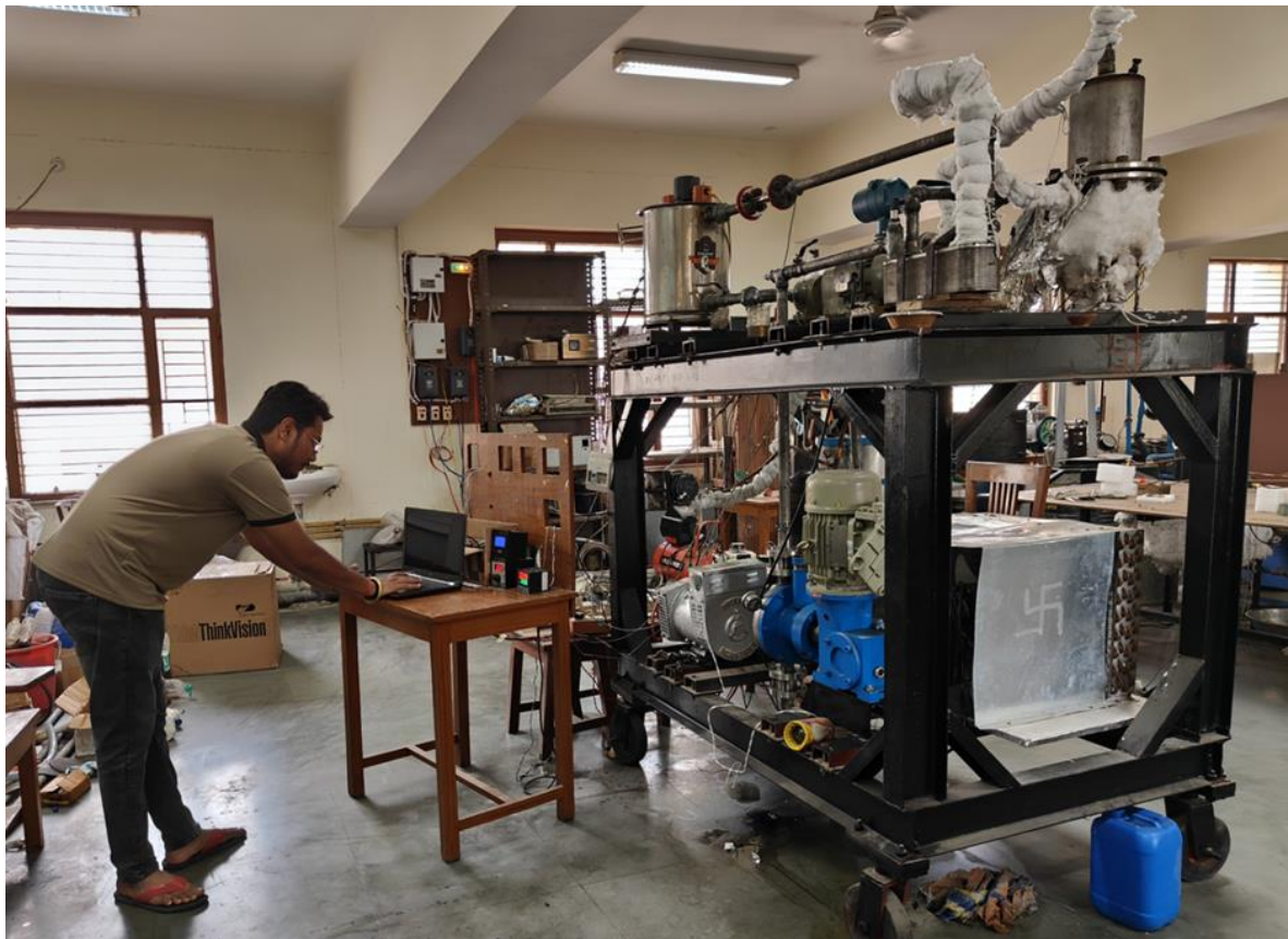
Figure 4.6. Isometric view and running condition of ORC experimental setup
