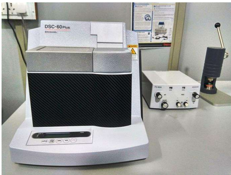
Figure 2.5: Experimental setup of DSC at Central instrument facility (CIF) IIT (BHU)
