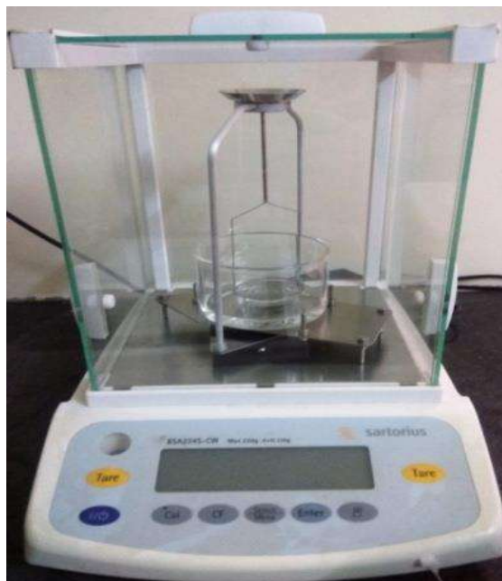
Figure 2.12: Density measurement kit by Sartorius, BSA2245-CW
