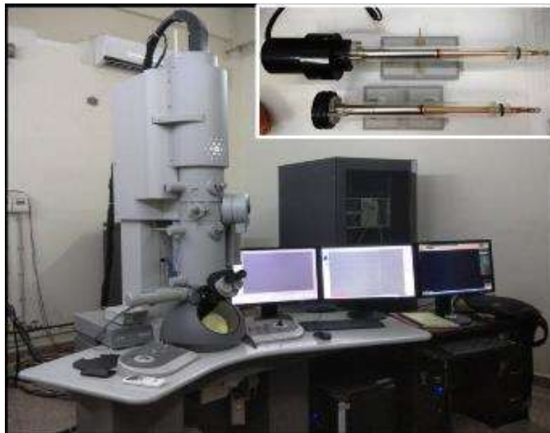
Figure 2.8: Experimental set up of the TEM technique at CIF-IIT (BHU), inset shows the sample holder
