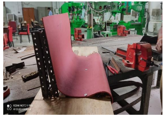
Figure 9.7: An adjustable prototype seat for measuring the weaver's seating shape
