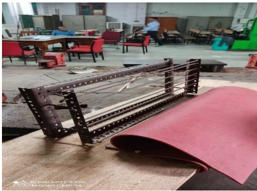
Figure 9.7: An adjustable prototype seat for measuring the weaver's seating shape
