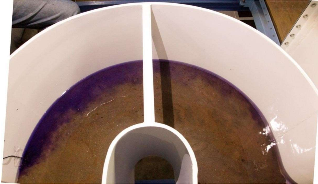
Figure 7.9 Pollutant Flow Pattern in Lab Channel
