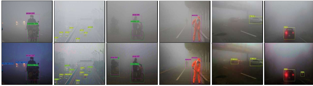
Figure 4.12: Object detection results on hazy images and their corresponding dehazed images (Top row - hazy images and bottom row - dehazed images).
