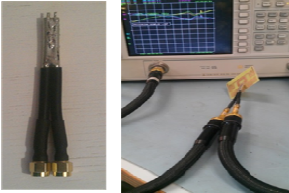
Figure 3.10: Differential probe with measurement setup
