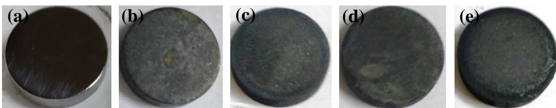
Fig. 6.12: Digital photographs of the disc samples exposed to oxidation at 850°C for various durations: (a) as polished (b) 50 h (c) 100 h (d) 500 h and (e) 1000 h.
