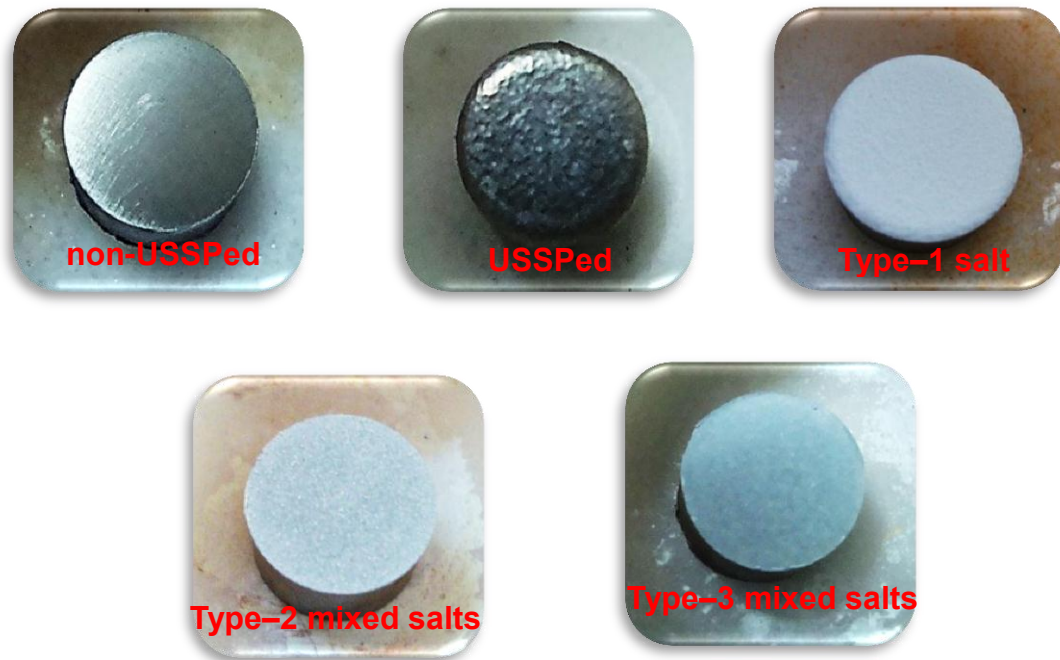
Fig. 5.1 Digital photographs of the non-sprayed and salt/mixed salts sprayed samples prior to exposure at elevated temperatures.
