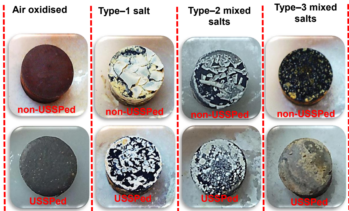
Fig. 5.4 Digital photographs of the non-USSPed and USSPed samples exposed at 600 °C for 100h.
