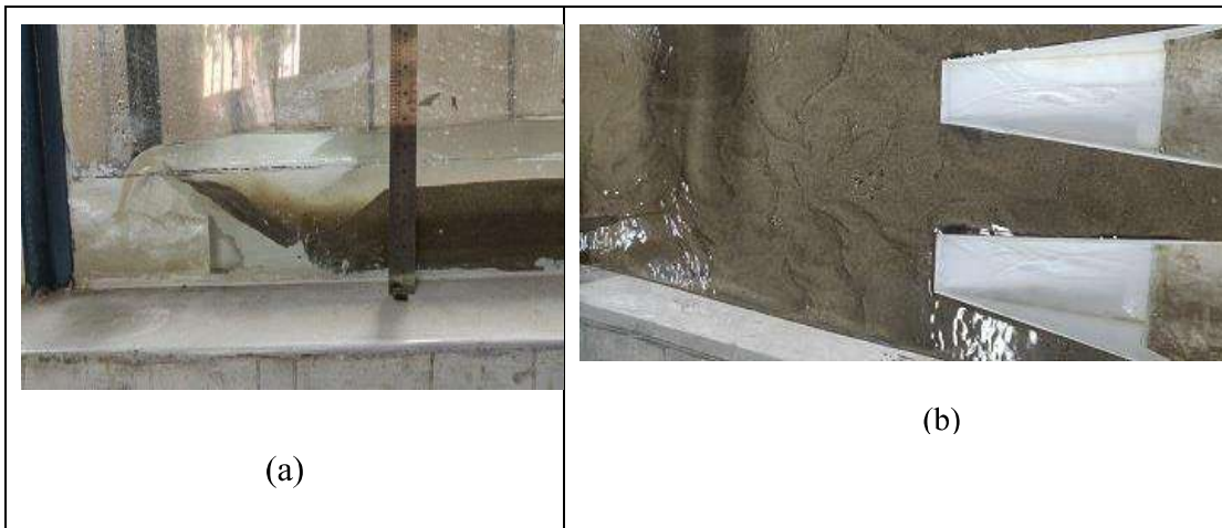
Figure 5. 8 (a) High degree of sediment uplift near the start of the inlet key and (b) Sediment passage beginning under the upstream overhang near the lateral crest
