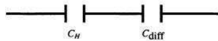
Figure 1.17: Equivalent circuit diagram of Cdl in Stern model [46] (Figure is taken from open access internet source)
