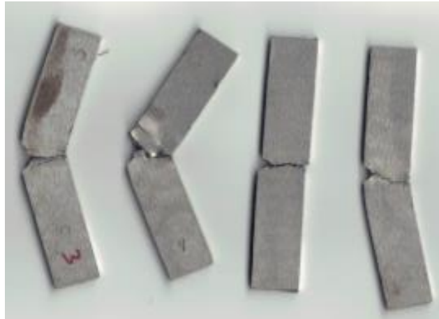
Figure 4.46 Charpy impact toughness test specimen after testing.
