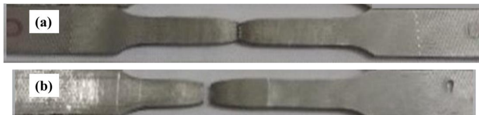
Figure 4.16 Transverse tensile test specimen after testing: (a) base metal, and (b) welded plate.
