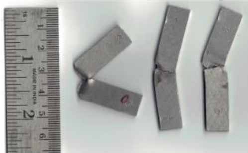
Figure 4.20 Charpy impact toughness test specimen after testing.
